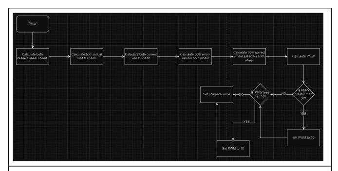
This is the Wheel Speed Control or the PWM function.
